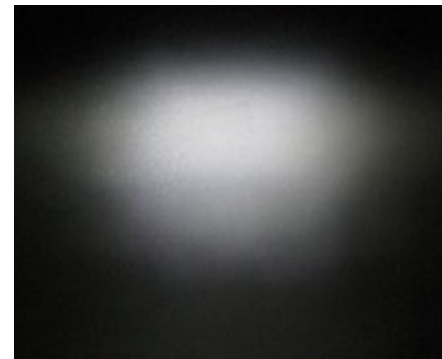
Shaped beam pattern: flat top, with sharp cutoff. Brightness tapers down toward the bottom for even illumination closer to the bicycle.
